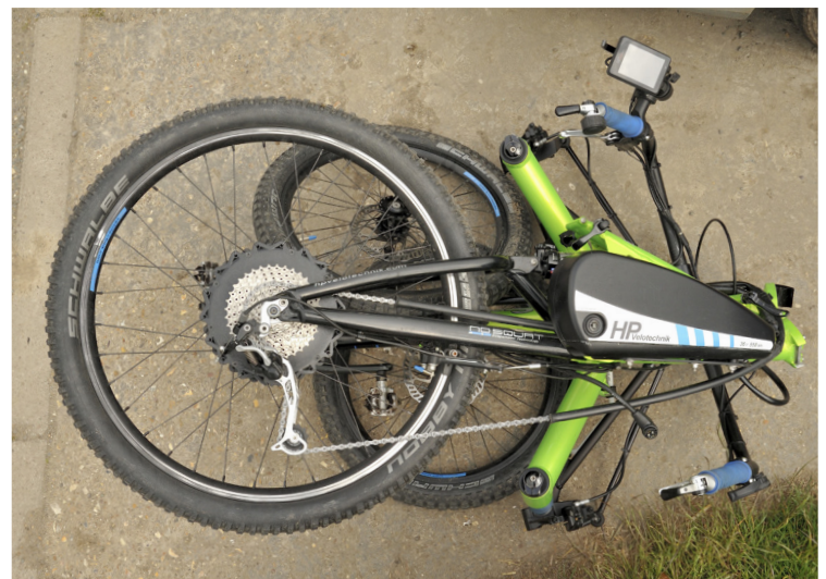
RIGHT: Trike, with wheels also removed and tucked below. The display looks vulnerable but could be protected by rotating the arm.
