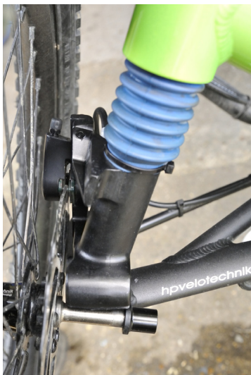
ABOVE: Fast one-key wheel removal.
