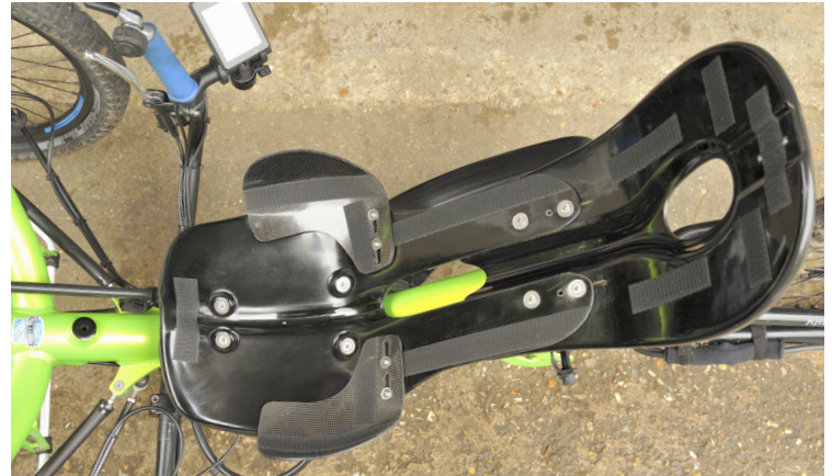
ABOVE: BodyLink seat with wings, Airflow pads removed.
